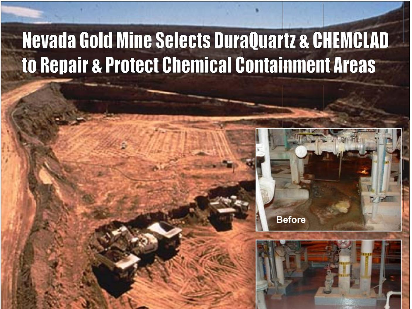
This concrete containment area was severely damaged by the strong chemicals used to strip gold from carbon ore. The chemical attack problems were exacerbated because the floor was pitched away from drains causing the chemicals to pool in certain areas.
